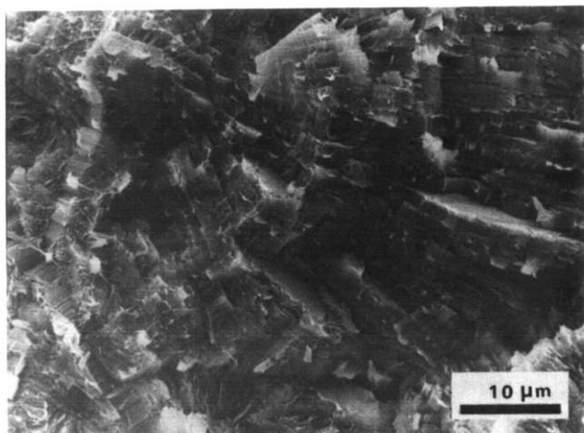
**Figure 1** Scanning electron micrograph of fractured surface of polyethylene crystallized at 0.6 GPa and 260°C for one day
