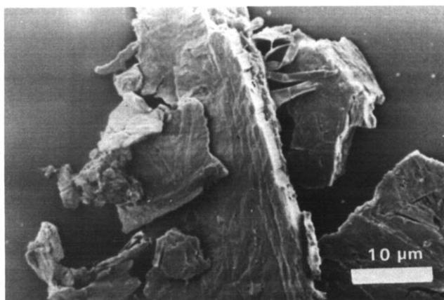
**Figure 2** Scanning electron micrograph of fragments of polyethylene. The sample was roughly broken and ultrasonically dispersed after the fuming nitric acid treatment
