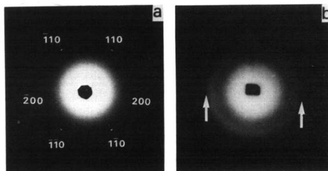
**Figure 4** (a) X-ray diffraction pattern of a single crystal of polyethylene crystallized under high pressure. The sample was oscillated around the vertical axis in *Figure 3*. Inner reflection of each 110 reflection is due to  $\text{CuK}\beta$  radiation. (b) X-ray diffraction pattern of the same sample as in (a). The sample was oscillated around the axis perpendicular to the end surface of the plate in *Figure 3*
