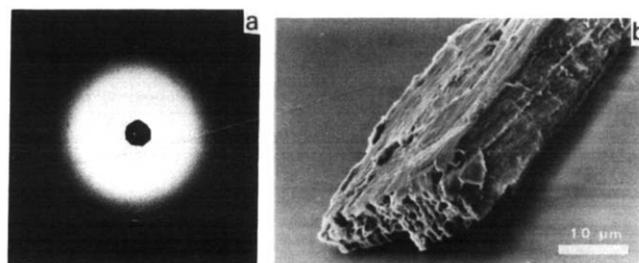
Figure 8 (a) X-ray diffraction pattern of a bulky polyethylene fragment. (b) A scanning electron micrograph. This fragment is made of several sheets of bands overlapped
