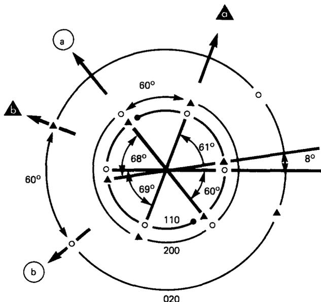
Figure 7 Reciprocal lattice construction for Figure 6b. There are two crystals; (○) represents the reciprocal lattice points of one single crystal and (▲) represents those of the other single crystal. The arrows drawn by thick line represent the *a*- and *b*-axes of the two crystals
