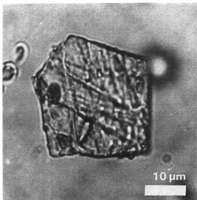
**Figure 3** Optical micrograph of a single crystal of polyethylene crystallized under high pressure
