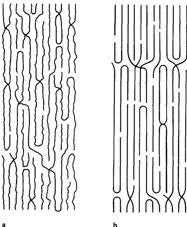
**Figure 10** Model for the phase transition of polyethylene from the hexagonal to the orthorhombic phase. (a) In the hexagonal phase, there are many defects along *c*-axis (kinks, jogs). (b) On the phase transition, these defects are excluded to form boundaries between bands
