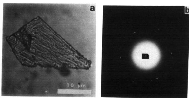
Figure 6 (a) An optical micrograph of a fragment composed of two single crystals. (b) X-ray diffraction pattern
