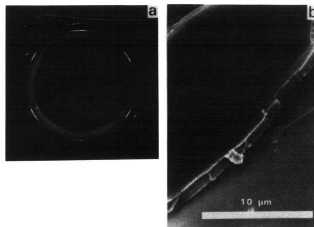
Figure 9 (a) An X-ray diffraction pattern of a band more than 0.1 mm wide. (b) A scanning electron micrograph of the fractured portion
