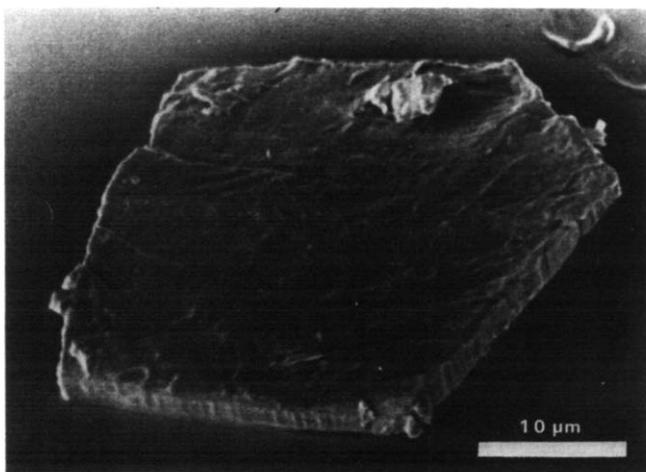
Figure 5 A scanning electron micrograph of a single crystal of polyethylene crystallized under high pressure
