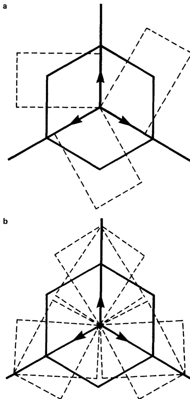
**Figure 11** Schematic representations for the possible orientations from the hexagonal to the orthorhombic phase. (a)  $\langle 100 \rangle_{\text{hex}} \rightarrow \langle 010 \rangle_{\text{orth}}$ ; (b)  $\langle 100 \rangle_{\text{hex}} \rightarrow \langle 110 \rangle_{\text{orth}}$ .
